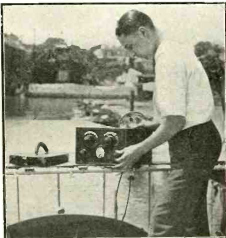
AL ODORF, operating the 6-tube Super-heterodyne he built, pictured also above. (Kadel & Herbert.)
